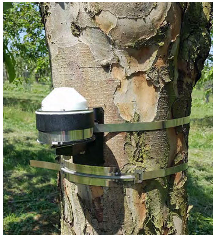
Figure 19. Automatic (top) and manual (bottom) band dendrometers installed on the trunk of an apple tree.
