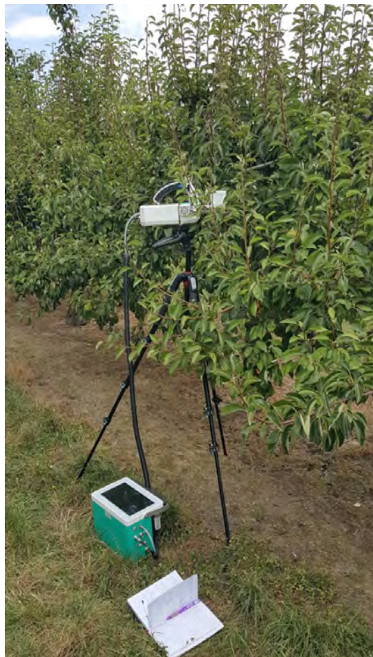
Figure 18. Measurement of air conductivity, photosynthesis, and transpiration with an infrared gas analyzer (LI-6800).
