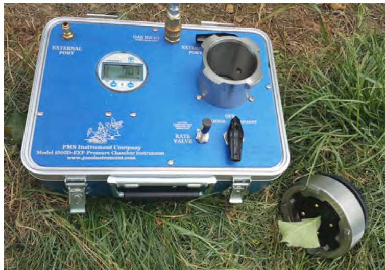
Figure 16. Scholander pressure chamber for water potential measurement. At lower right, a leaf is fixed in the lid of the pressure chamber.
