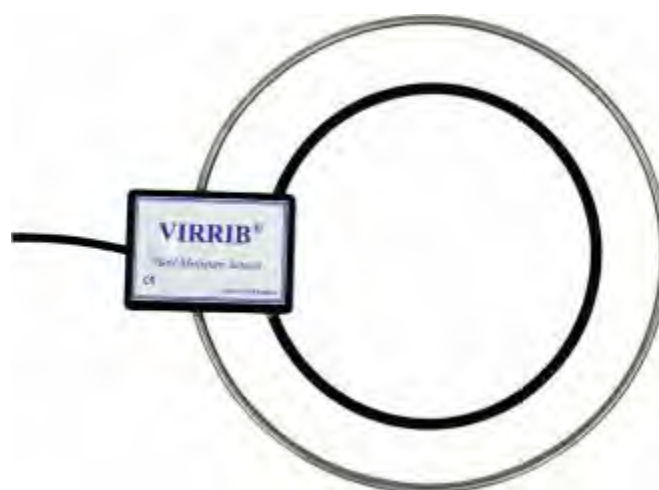
Figure 4. Soil volumetric moisture sensor VIRRIB (product of AMET, Velké Bílovice)
